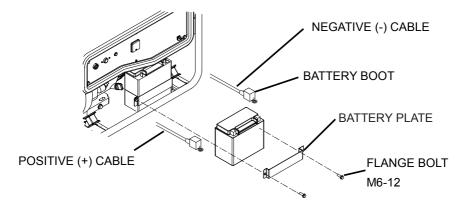
5. Install the battery. Install battery plate using two M6-12mm flange bolts.
